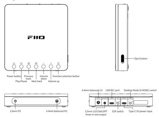
**Power button:** Long press to turn on or off. When powering on, short press the power button to check the power and working status. For example, BAT4 represents the battery level is 80%-90%. The other status it will also display at the same time.
